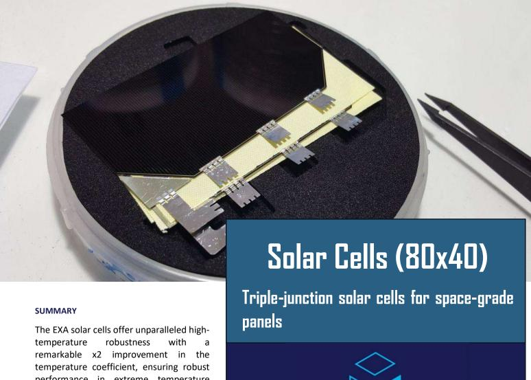
performance in extreme temperature variations. EXA's solar cells achieve ultrahigh efficiency and a lightweight design of 80-120 mg/cm<sup>2</sup>, boasting an impressive efficiency of >30% and >27% (AM v 1.5, outdoor).
